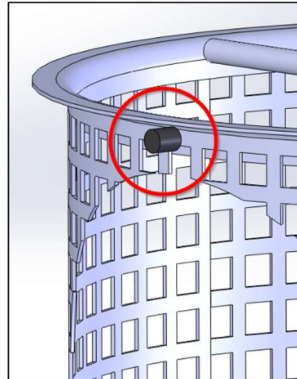
Figure 2 How to fit strainer.
