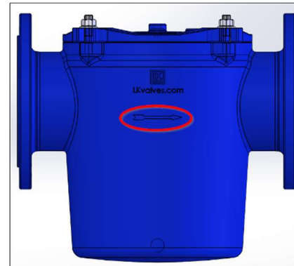
Figure 7 Arrow displays flow direction.
